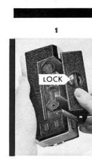
cover lock clockwise, as far as it will go  $(\frac{1}{4}-turn)$  to secure it in place. Check to make certain that the cover is fastened.
